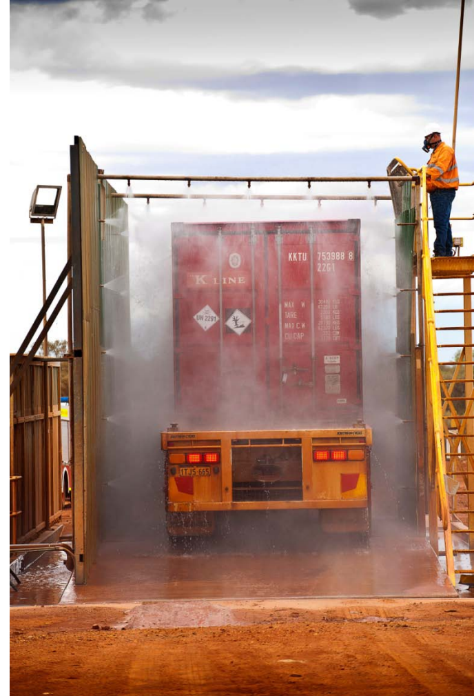
Truck being washed before leaving site
