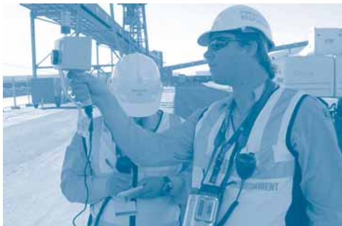
DEC officers use a hand-held dust monitor to test air quality at the Esperance port.
